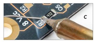
Allow the resistor to cool for a moment, then solder the other end of the resistor in place (C). When you are done, you should have a neat meniscus of solder on both ends of the resistor (D), bonding it neatly in place.
