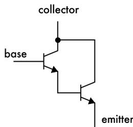
In the Darlington configuration, the emitter of one transistor is connected to the base of another. This effectively makes one new “super transistor” out of the two, since it is the amplified current out of the first collector that serves as the base current for the second transistor. If the gain of a single transistor were 30, then the effective gain of the Darlington pair would be  $30 \times 30 = 900$ .
