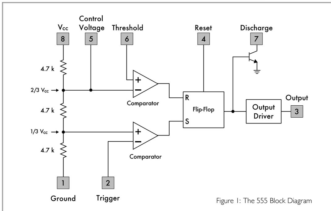
Figure 1: The 555 Block Diagram
