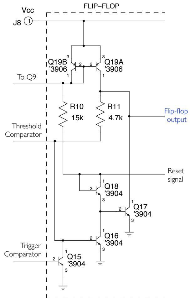
Figure 7: Flip Flop Block
