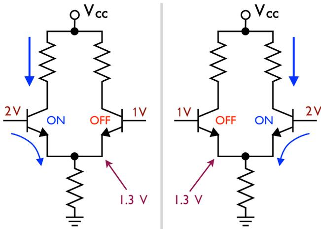
Figure 4: Simplified differential amplifier
