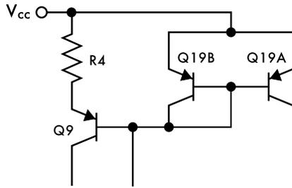
Current mirrors can be constructed with multiple “output” transistors, and Q9 is an additional output transistor that – in parallel with Q19A – tracks changes in the current through Q19B.
