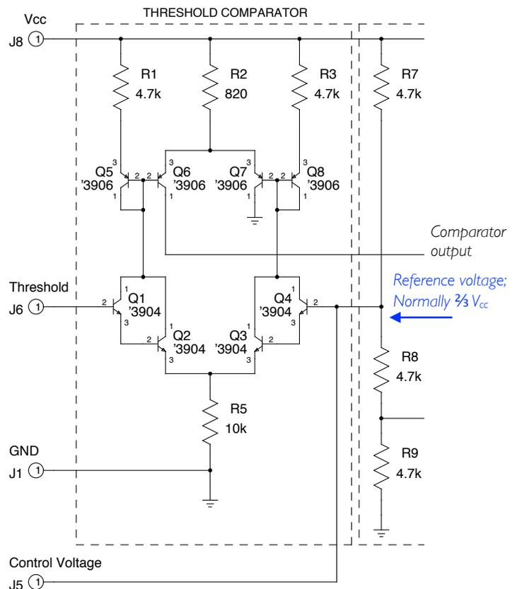
Figure 3: Threshold Comparator
