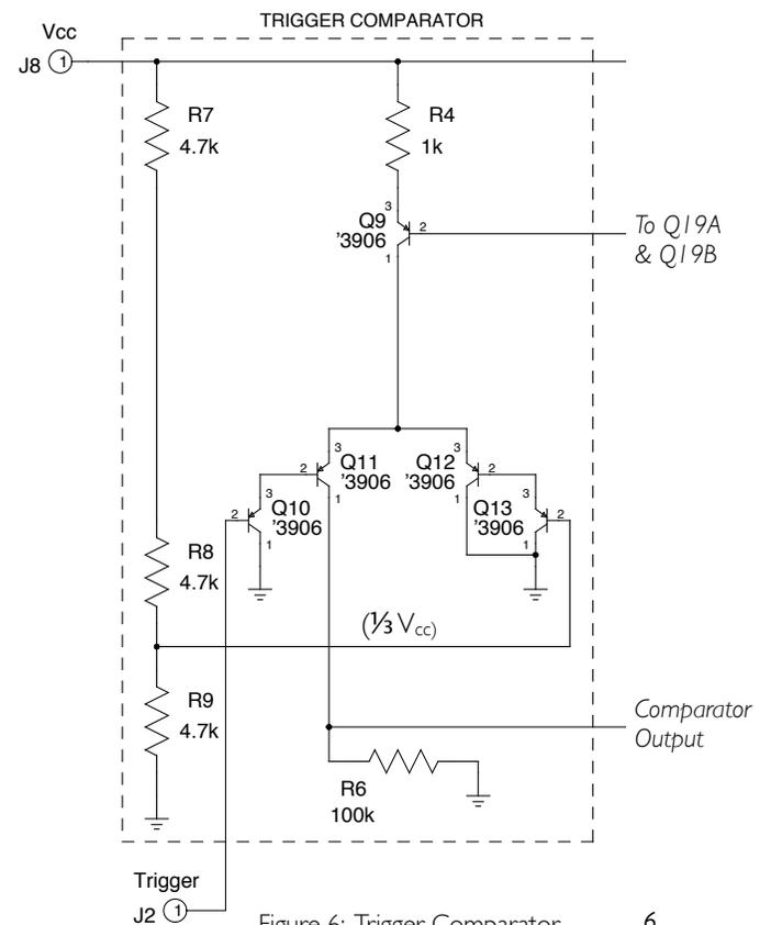
Figure 6: Trigger Comparator
