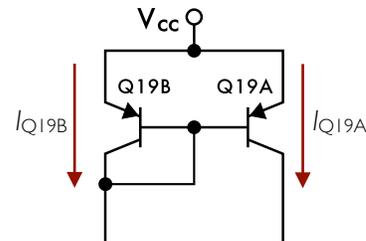
Figure 5: Q19A/Q19B Current Mirror
