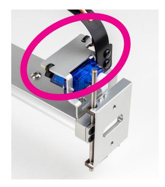
(B) If the mounting bracket looks like the photo above, with a silver-colored aluminum flap that covers the top of the servo motor:
