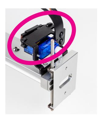
(A) If the mounting bracket looks like the photo above, with a **black-colored** aluminum flap that **covers the top** of the servo motor:
